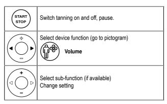
Pictograms of available functions are illuminated in default mode after starting up the sunbed. After selecting a function, the corresponding pictogram and the navigation ring flash for a short time. During this time settings may be changed.
